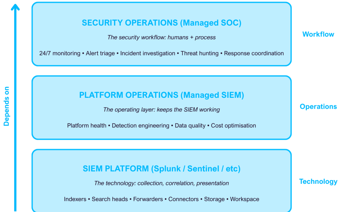
Figure 3. Two distinct layers. A Managed SOC handles the security workflow. A Managed SIEM handles the platform operations the SOC depends on.
